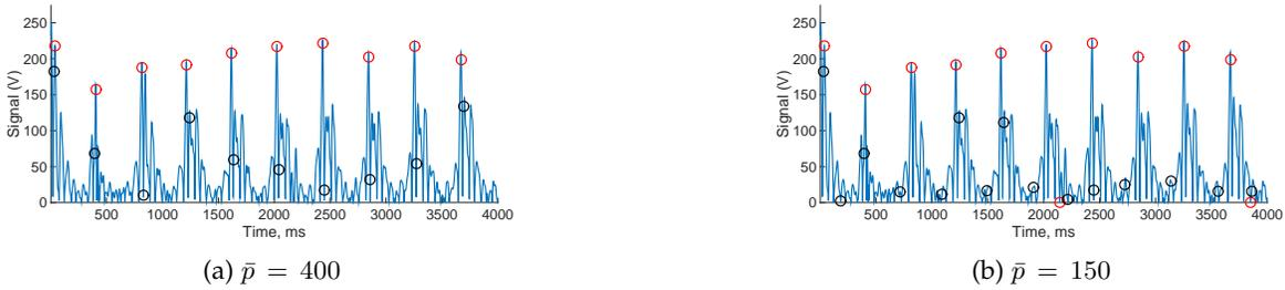
Fig. 3: peakWPM-detected peaks (red circles) and peakWPB-detected peaks (black circles) on a VT rhythm.
